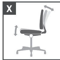
X. Dual-clutch posture control — Adjusts seat and back angles independently with two levers (infinite locking within a fixed range).
