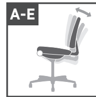
A-E. Back reclines at a 2 to 1 ratio to seat angle. Back angle adjusts independently of seat and can be locked in infinite number of positions within a fixed range.
